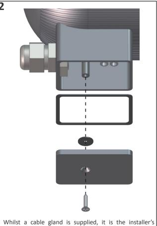
Whilst a cable gland is supplied, it is the installer's responsibility that it is both fitted correctly and suitable for the supply cable in use.
