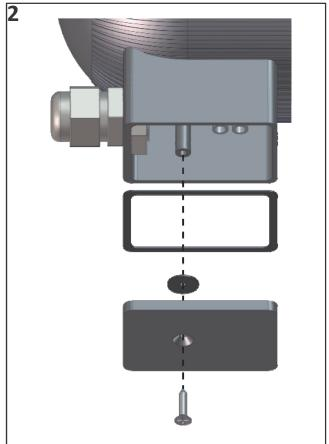
Whilst a cable gland is supplied, it is the installer's responsibility that it is both fitted correctly and suitable for the supply cable in use.
